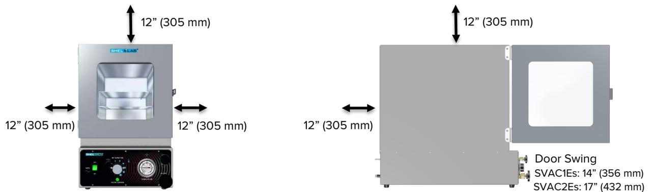
**12 inches (305 mm)** of clearance is required on the sides and back.
