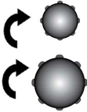
Check that oven chamber door is closed and latched, and that the vent and vacuum valves are both in the closed position.
