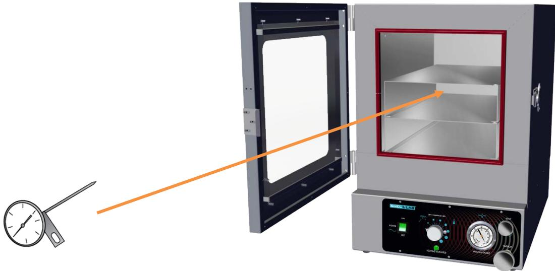
1. Place the thermometer on the top shelf of the oven where the face will be visible through the glass door.
