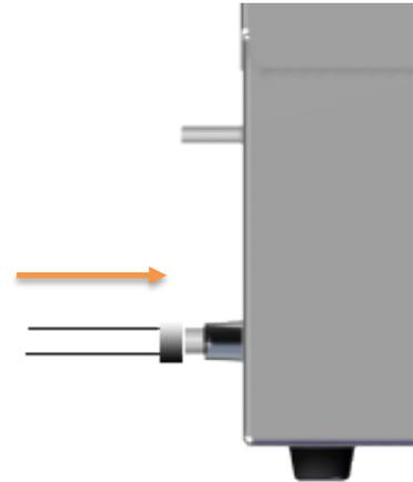
**Figure 4:** Vacuum Line Connected to Vacuum Port
